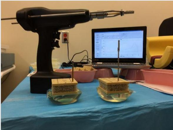
**Figure 2.** Plunge models showing essentially no plunge with VDC drill on left; plunge model to right with Standard drill and 10 mm plunge.
